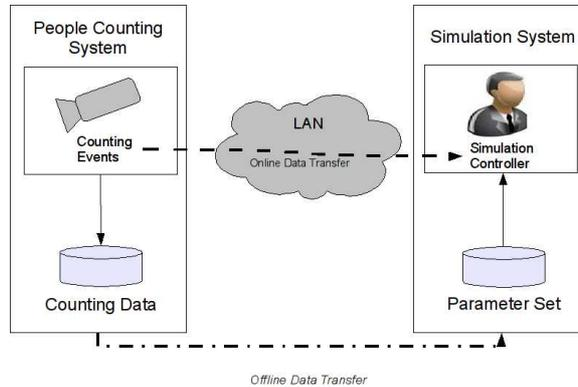
**Fig. 5. System layout and online/offline data transfer**
