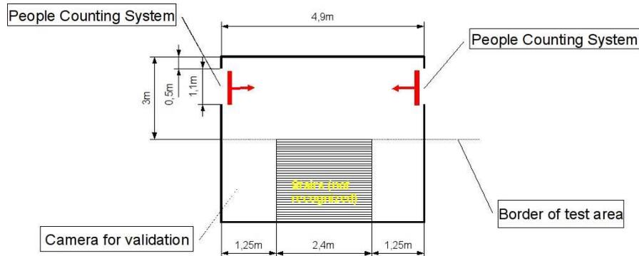
**Fig. 6. Laboratory setup for test data acquisition**
